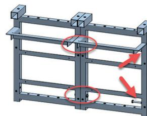
5. Secure the beams with bolts
