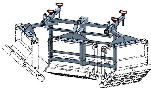
The modular mount for crane lighting is impressive with its simplicity, durability and expandability. It can be fitted on the ground by one person ready for use, and be to the crane. It can be also dismantled into its separate modules, which have been designed to save space.
