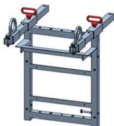
9. To position the middle lights optimally, "central lighting bracket" can be applied
